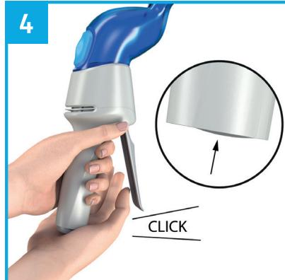
... and push the piercing element **F** up completely into the handle **D** until you will hear a click.
